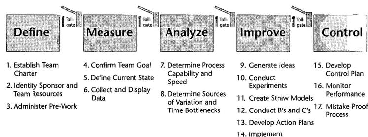
Figure 10-1. The DMAIC process
