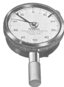
FIGURE 9-47 The maximum reading hand is a convenience for indicating the maximum value of a fluctuating variable, such as checking eccentricity or runout. Obviously, it could be a serious cause for error if the total travel required is more than one revolution. (Courtesy of Federal Products Corp.)
