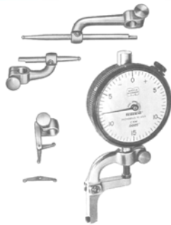
FIGURE 9-49 Right angle attachments permit the indicator to be located for best viewing position. Various types are shown at the top and bottom left. For permanent setups, the perpendicular indicators are preferred. (Courtesy of Federal Products Corp.)
