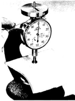
FIGURE 9-45 Weights are used instead of pull-back springs when gaging pressure must be constant and a stipulated amount. This is required when measuring compressible materials. A wide, flat contact point is usually required as well. (Courtesy of B. C. Ames Co.)
