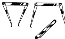
Combination calipers provide for a large range of inside and outside measurements.
