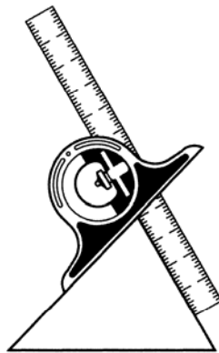
FIGURE 5-22 The protractor head with sliding blade forms a versatile instrument for the measurement of angles.
