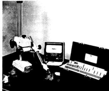
FIGURE 10-44 Height gage setups use a surface plate or the part itself as a reference surface.
