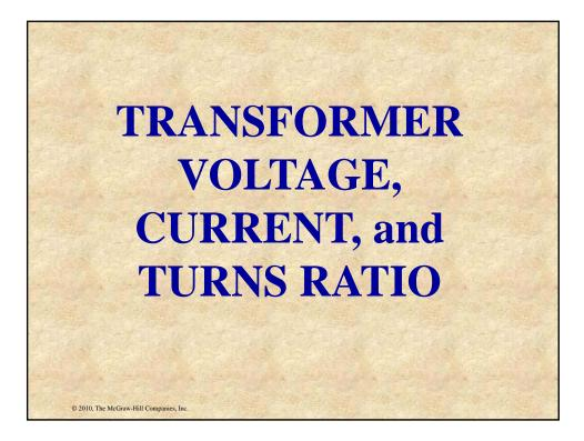
The ratio of turns in a transformer's primary winding to those in its secondary winding is known as the *turns ratio* and is the same as the transformer's *voltage ratio*. The voltage ratio of an ideal transformer (one with no losses) is directly related to the turns ratio, while the *current ratio* is inversely related to the turns ratio.
