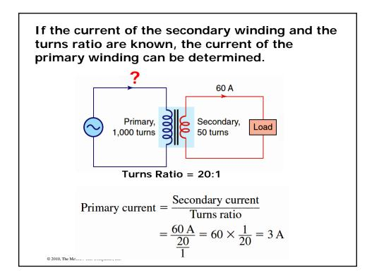
A transformer automatically adjusts its input current to meet the requirements of its output or load current. If no load is connected to the secondary winding, only a small amount of current known as the *magnetizing current* or *exciting current* current flows through the primary winding.
